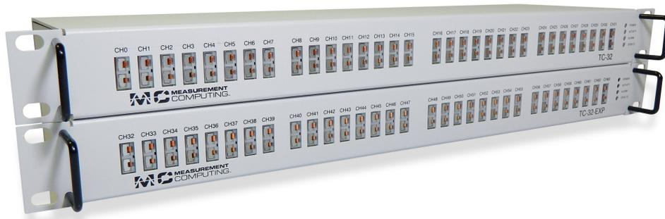
A TC-32 connected to a TC-32-EXP device provides up to 64 TC inputs, 16 digital inputs, and 64 digital outputs which can be configured as alarms. All DIO channels are isolated.
