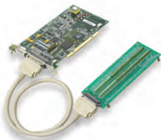
DaqBoard/3000 attached to a TB-100 terminal board
