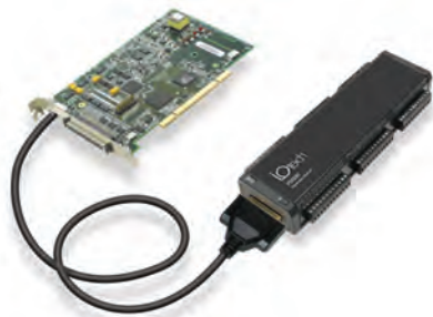
DaqBoard/3000 attached to a PDQ30 expansion module
