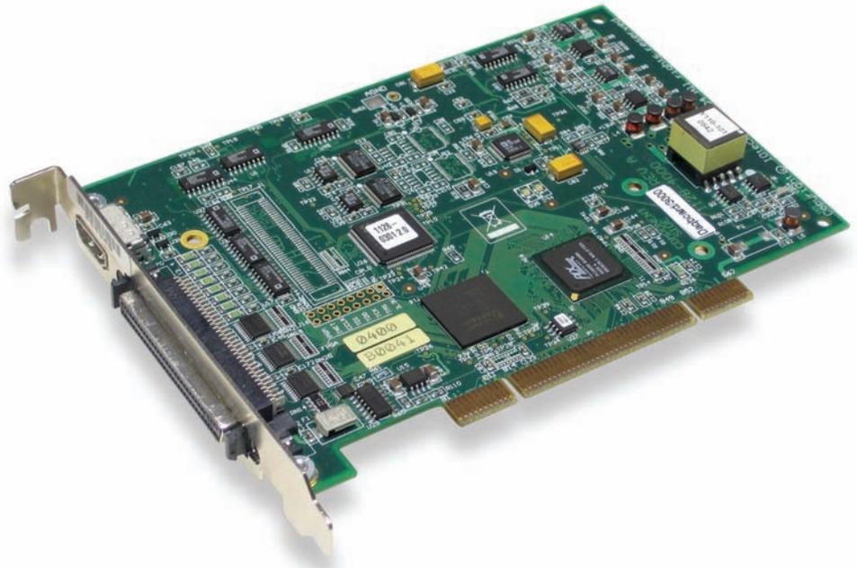
The PCI-2500 Series provides 1 MHz sampling, synchronous multifunction I/O, analog input expansion capability, and extensive software support
