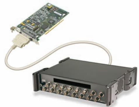
PCI-2500 attached to a DBK215 BNC and screw-terminal module
